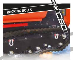
the machine's undercarriage, unique to the Cormidi line, has suspensions follow the terrain profile for increased stability and comfort.
